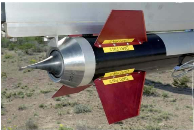
NASA Dryden Flight Research Center Photo Collection http://www.dfrc.nasa.gov/Gallery/Photo/index.html NASA Photo: EC04-0113-146 Date: March 30, 2004 Photo By: Carla Thomas A closeup of one of the Cesaroni Technology, Inc. - constructed aerospike nozzles used in the Dryden Aerospike Rocket Test.
