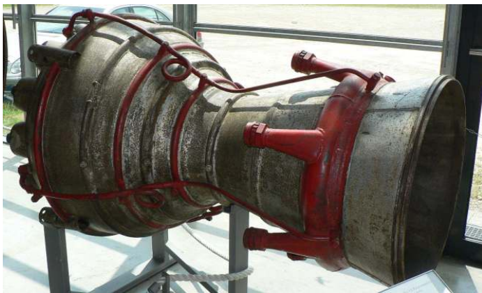
De Laval convergent-divergent nozzle from a V2 rocket motor
