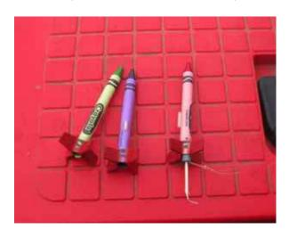
So, what do you need to build real crayon rockets? Well, real crayons, of course, and a ¼ inch drill. Add to that a little balsa wood, a launch lug, some paint and glue and you are there. Get a whole box of crayons as you are going to screw up a few figuring out how to drill a Micro Maxx sized hole in a crayon that is just slightly larger in diameter than the engine.
