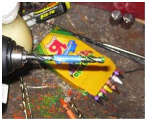
I tried drilling a larger hole that would fit a Micro Maxx engine tube, but there was just not enough crayon left after the drilling so I had to forgo the engine mount and insert the Micro Maxx directly into the wax. I was a little concerned that the heat of the engine might melt the wax and cause problems, but it turned out to not be a problem.
