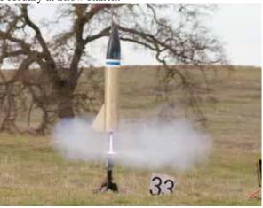
The motor is producing thrust, but you can see that the nose cone has already started moving forward (the blue stripe is masking tape)
